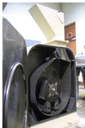
Fig. 1. Overhead view of hammer mill and instrumentation set up and picture showing hammers and classifying screen of hammer mill.
