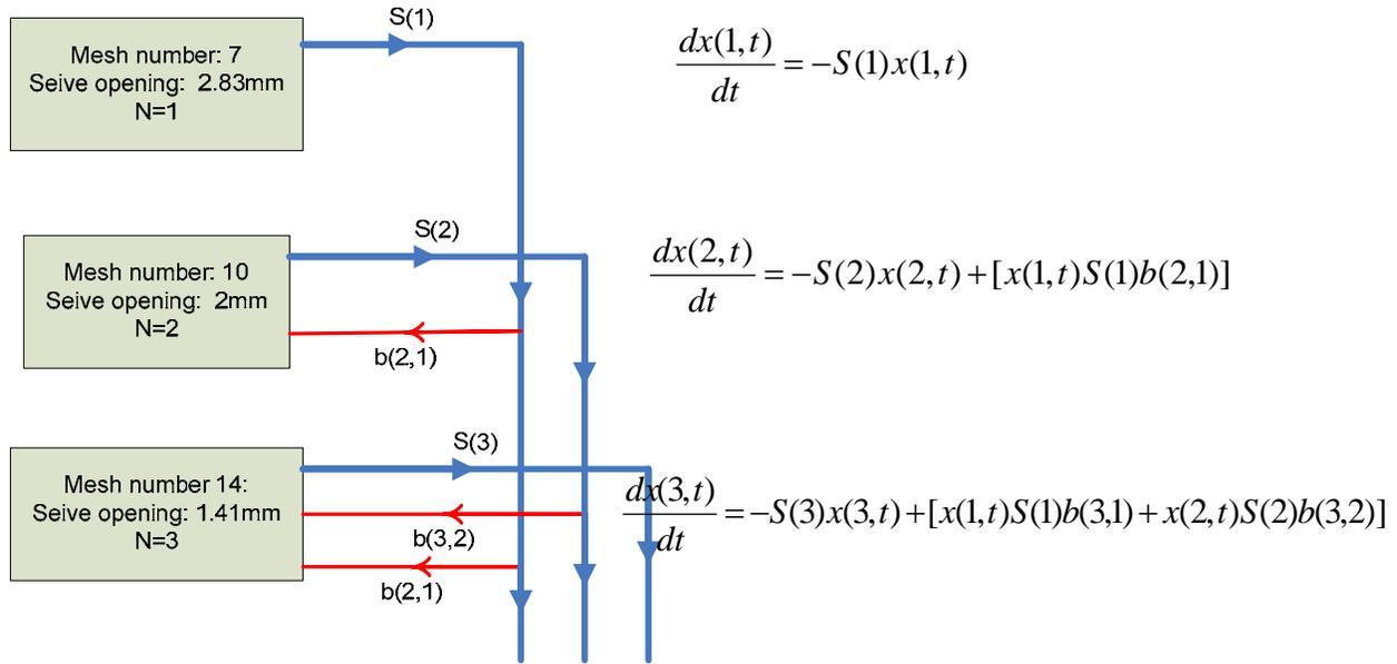
Figure 2. The simplified 3 steps of size intervals and the correspondent mass-rate balance.
