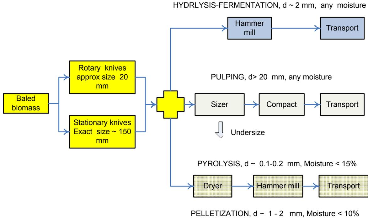
Figure 1. The overall ranges of particle sizes and equipment used to generate the sizes.
