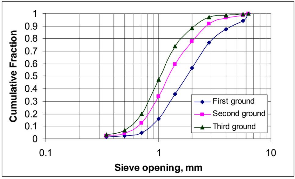
Figure 4 .Cumulative size distributions of the three grinds vs. sieve opening.
