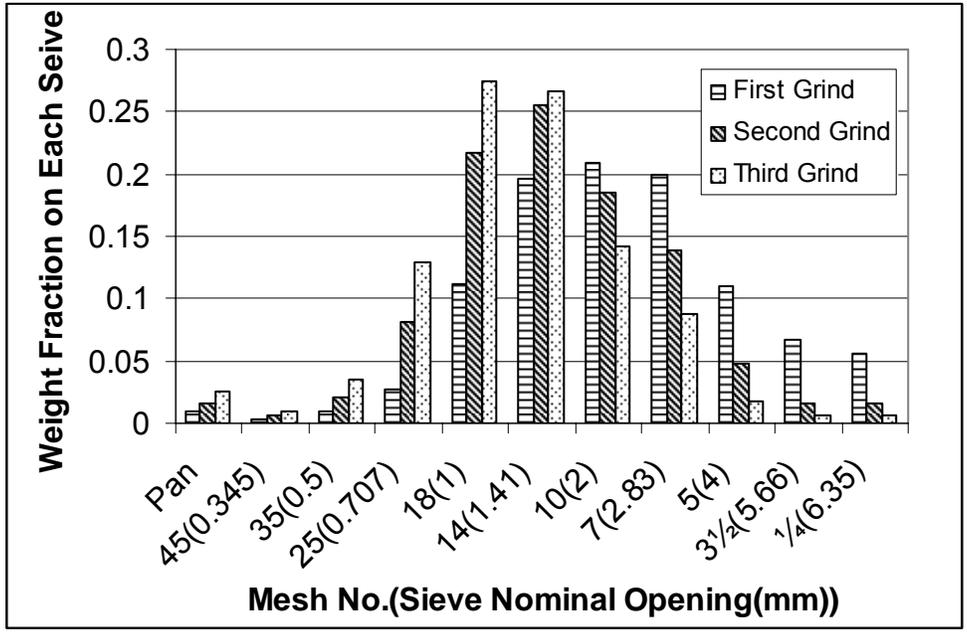
Figure 3. Size distribution of switch grass grind: Fraction vs. Mesh Number.
