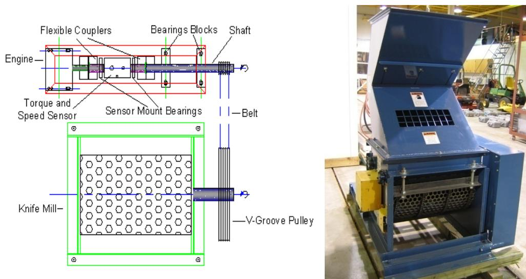
Figure 1. Overhead sectional view of knife mill and instrumentation set up and photo of knife mill.
