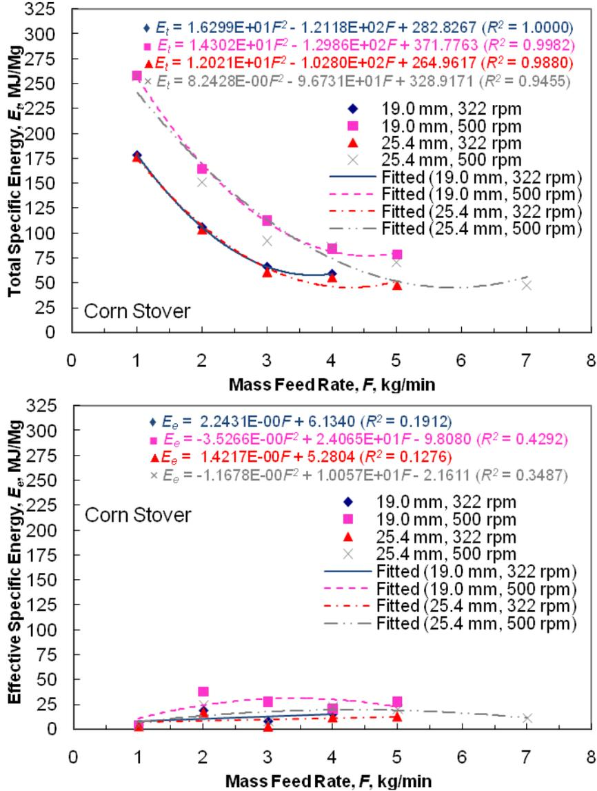
Figure 8. Total and effective specific energy of corn stover with knife mill mass feed rate at selected screen sizes and corresponding speeds sizes.
