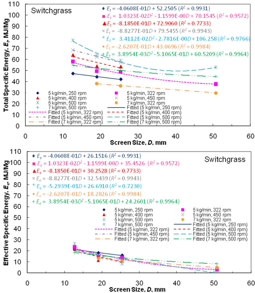
Figure 7. Total and effective specific energy of switchgrass with knife mill screen size at selected mass feed rates and corresponding screen sizes.
