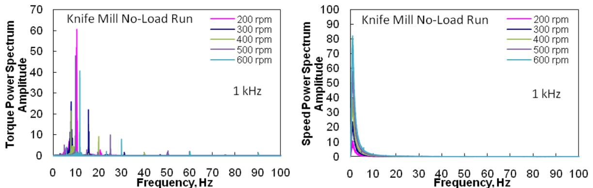
Figure 2. Power spectra of torque and speed for 1 kHz data acquisition sampling rates during no-load run of knife mill.
