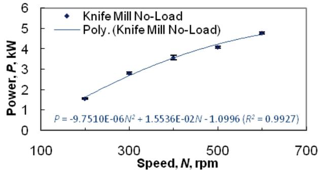
Figure 4. No-load power consumption of knife mill with speed.
