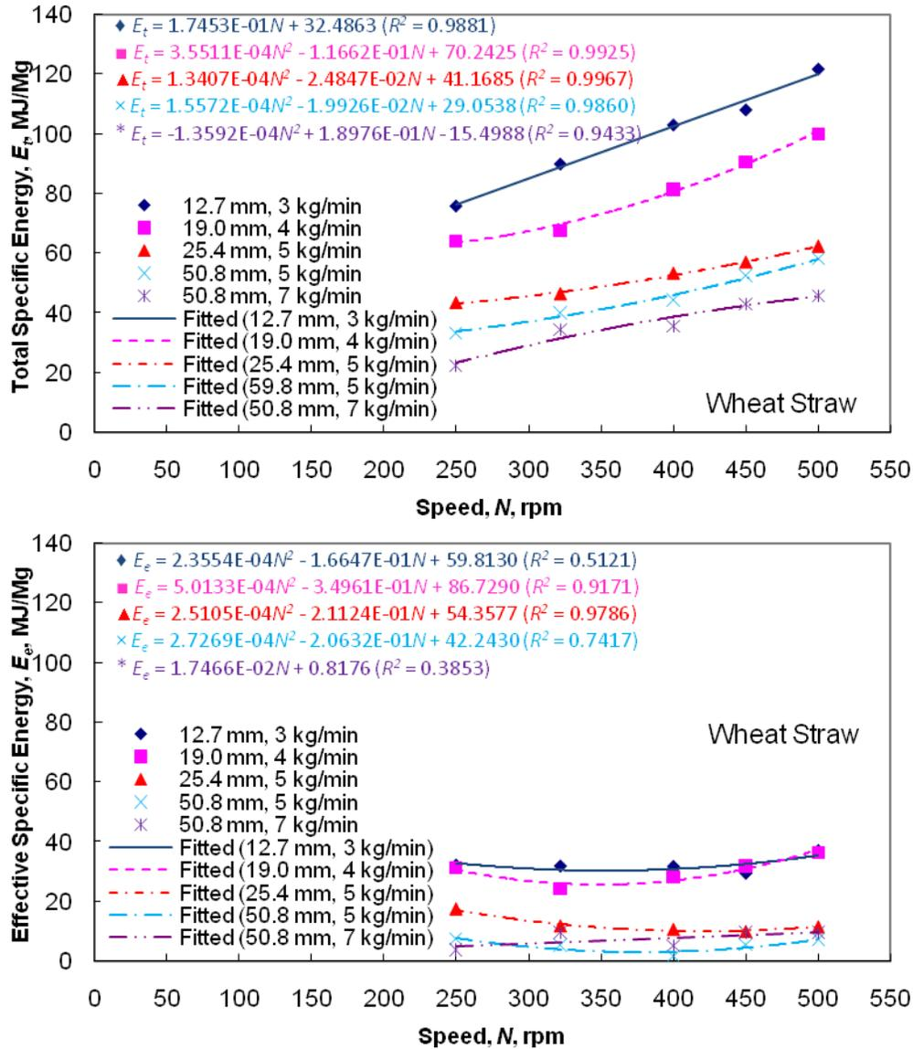
Figure 6. Total and effective specific energy of wheat straw with knife mill speed at selected screen sizes and corresponding mass feed rates.
