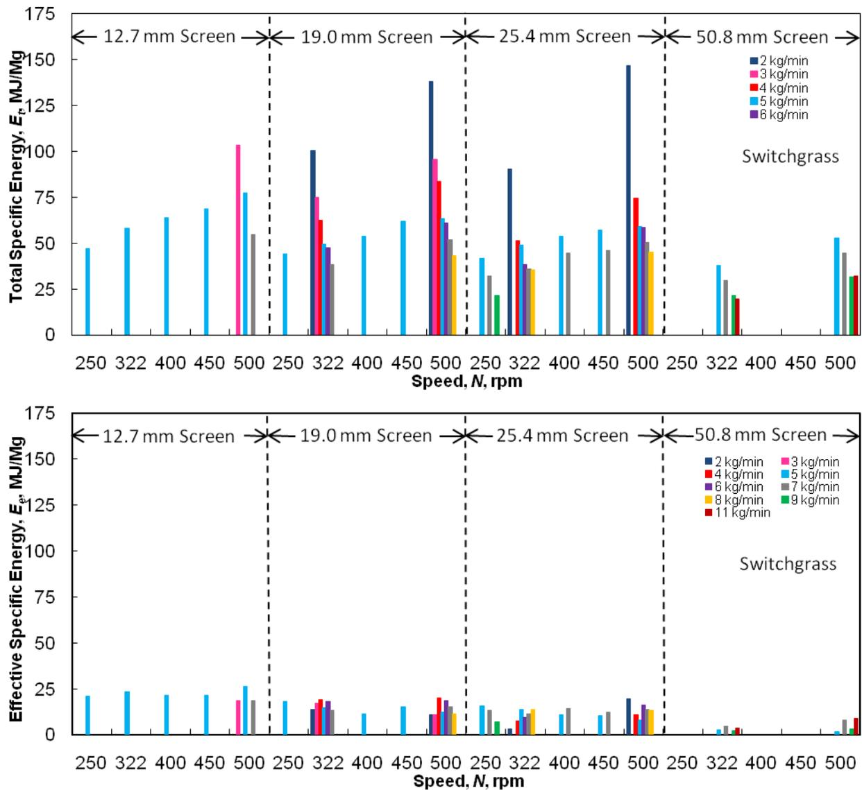
Figure 5. Total and effective specific energy of switchgrass with knife mill speed at various mass feed rates.
